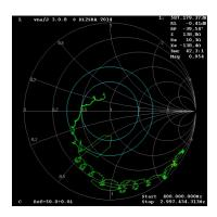
tinyVNA, circuit 1 400 ... 3000MHz Note the graph is very noisy, and only gives an impression of impedance.
